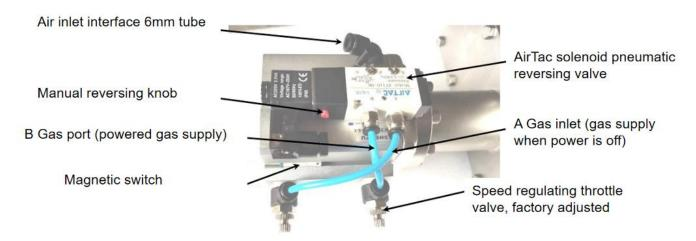
4. See the right picture for the wiring diagram of the valve magnetic switch signal. It can be connected to PLC or intermediate relay to realize automatic control.
